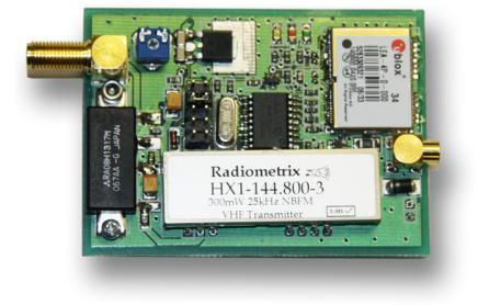
WARNING : DO NOT POWER UP THE UNIT WITHOUT AN RF ANTENNA
